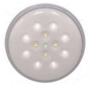
The 8 LED crown can be set at 5,700 K or 3,000 K to light when the Orión is on mains, if the maintained mode is chosen. For the crown not to light and the Orión is in non-maintained mode, a connector inside the Orión needs to be repositioned.
